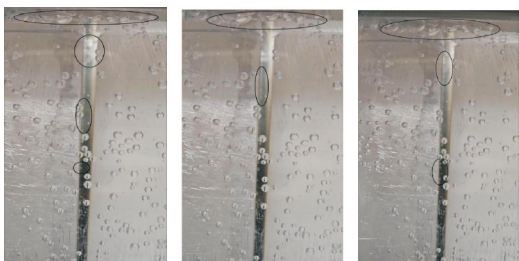
图9 4 C放电工况下氟化液沸腾情况 Fig. 9 Boiling condition of the fluorinated liquid under 4 C discharge condition
