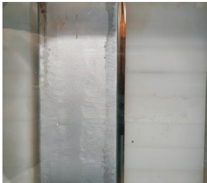
图7 1 C放电工况下电池箱氟化液状态 Fig. 7 Status of fluorinated liquid in the battery pack under 1 C discharge condition
